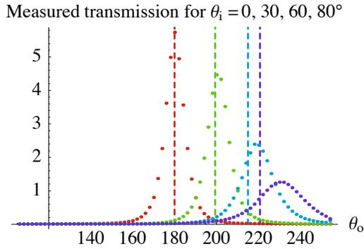
**Figure 2:** Measured transmission ( $f_t(\mathbf{i}, \mathbf{o}, \mathbf{n}) |\mathbf{o} \cdot \mathbf{n}|$ ) for a rough surface (ground glass) at 0, 30, 60, and 80 degrees incidence angle. Dashed lines are the refracted directions predicted by Snell's law for a smooth surface. Note that the transmitted lobe grows broader as the incidence angle increases and is shifted significantly towards grazing compared to refraction through a smooth surface.
