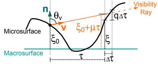
**Figure 16:** Geometry for Smith shadowing-masking  $G_1$  for direction  $\mathbf{v}$ , corresponding to a visibility ray has starting height  $\xi_0$  and slope  $\mu$ . At distance  $\tau$  (measured along macrosurface), the microsurface has height  $\xi$  and slope  $q$ .
