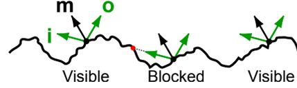
Figure 5: Shadowing-masking geometry: Three points with the same microsurface normal  $\mathbf{m}$ . Two are visible in both the  $\mathbf{i}$  and  $\mathbf{o}$  directions, while one is blocked (in  $\mathbf{i}$  in this case). By convention, we always use directions which point away from the surface.
