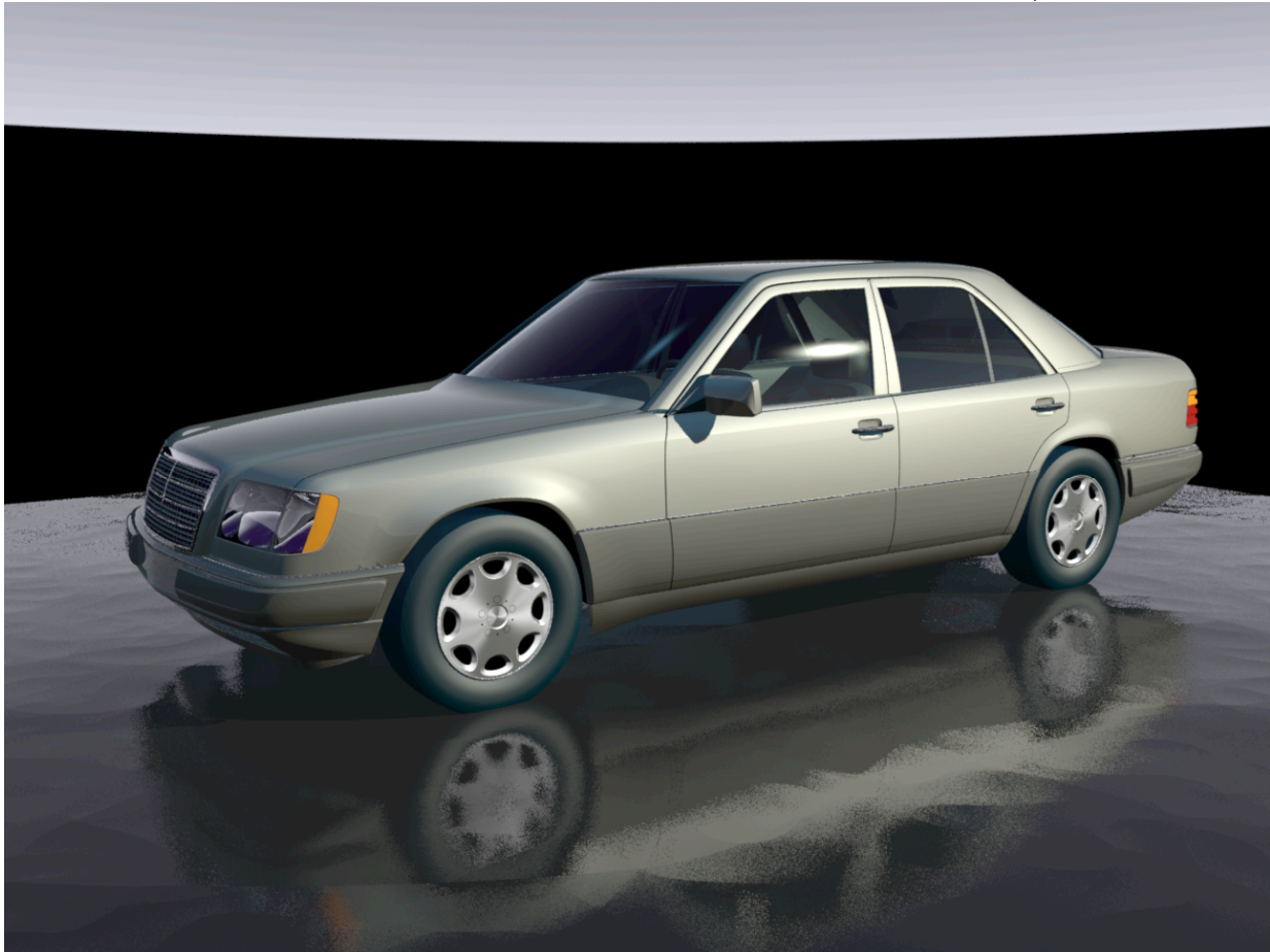
Figure 13. Computer-generated image based on measured BRDF of the metallic silver paint
