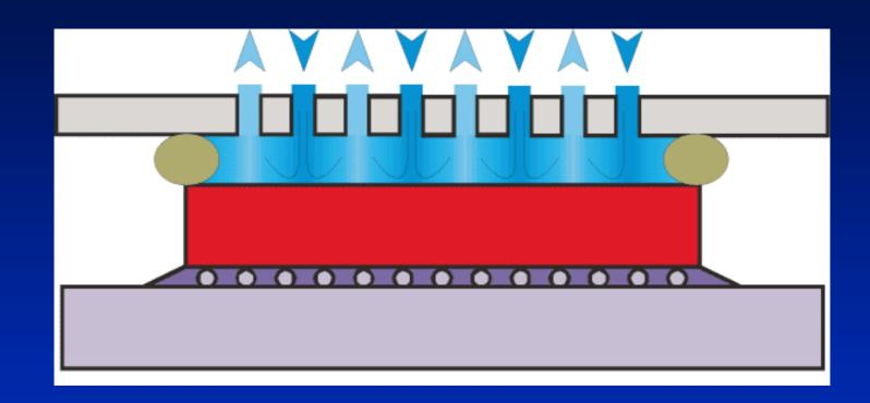
Distributed return architecture with cross section showing inlet jets with neighboring drainage holes.
