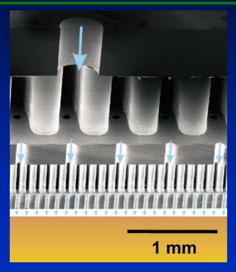
SEM section of two-level jet plate. Water flow is indicated by blue arrows.
