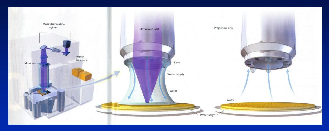
By adding a thin layer of water between the projection lens and the wafer, the immersion system can create features 30 percent smaller.
