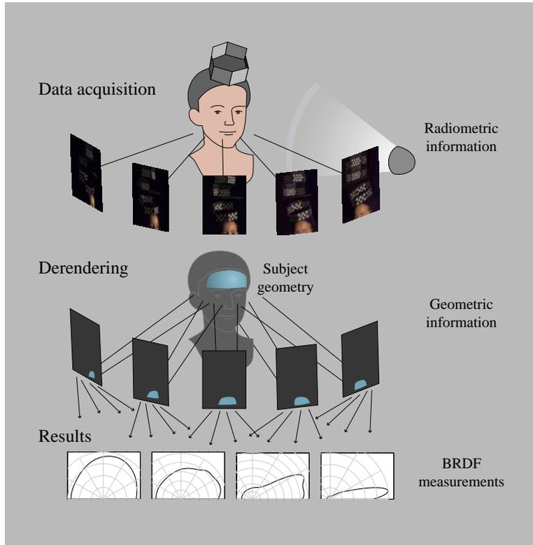
Figure 2: BRDF measurement process
