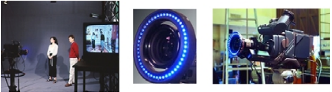
Figure 3.11: The BBC's LiteRing system uses low-powered, colored LEDs to illuminate a mesh screen, which then feeds a traditional linear keying process. The integral part of the system is the gray mesh, which is made up of millions of very small glass beads. These beads make the screen highly retroreflective, allowing it to reflect almost all incident light back to its source, independent of the angle of incidence to the screen. This retroreflectivity cause the background to take on the color of the LEDs, observable only from the lens' location. Images courtesy of Reflecmidia.
