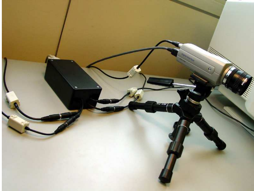
Figure 3.5: A DFW-X700 camera and the trigger circuit box.
