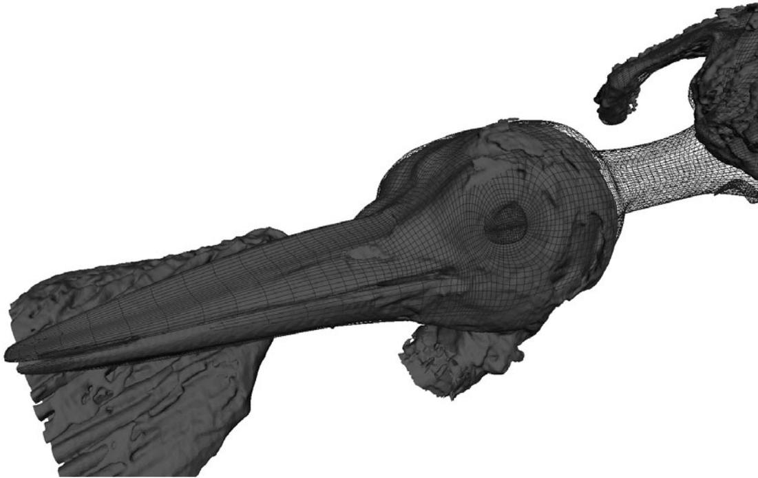
Figure 4.12: Comparison between the original reconstructed model (dark gray) and smoothed animation model (wireframe).
