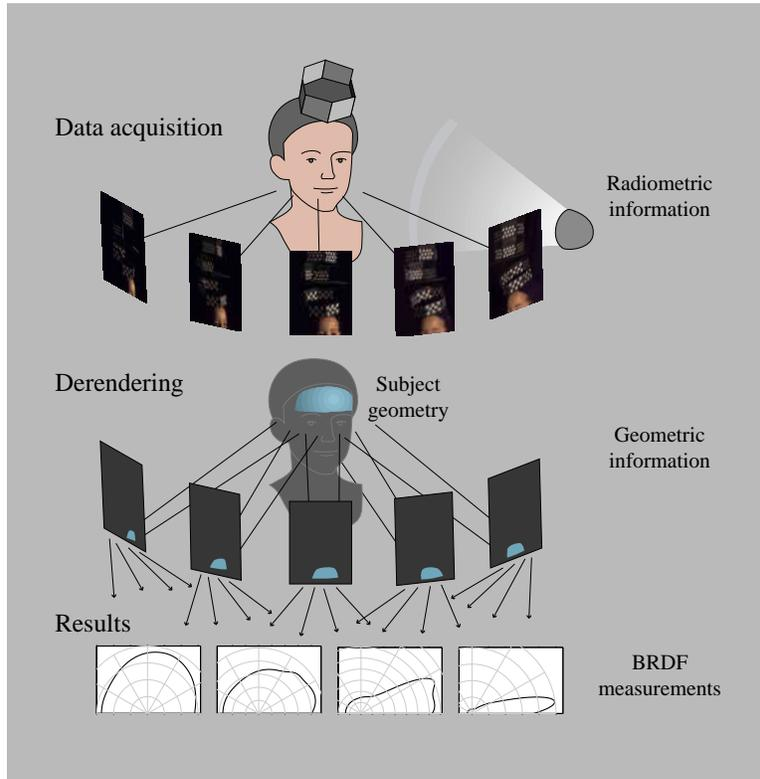
Figure 2: BRDF measurement process
