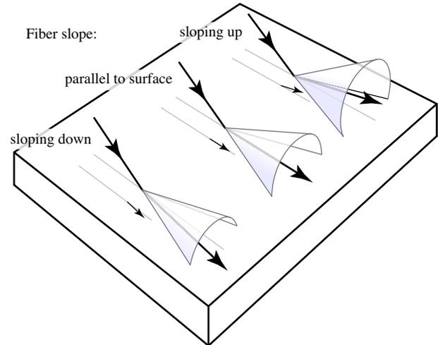
Figure 1: The basic shape of the *subsurface* reflection from fibers inclined downward, parallel to the surface, and inclined upward. Models for anisotropic *surface* reflection produce results similar to the center drawing.
