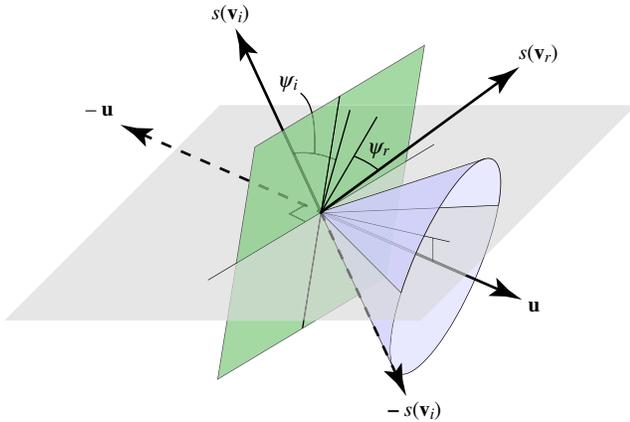
Figure 7: Geometry for fiber reflection model. Specular reflection from the subsurface fibers occurs when the refracted reflection direction,  $s(\mathbf{v}_r)$ , is in the cone centered on the fiber axis  $\mathbf{u}$  and containing the opposite of the refracted incident direction,  $-s(\mathbf{v}_i)$ .
